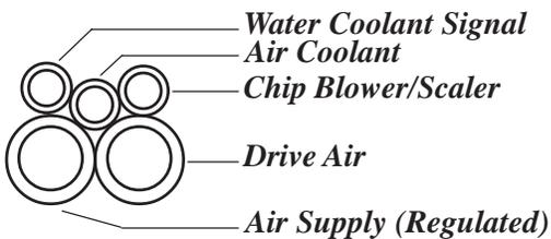
Figure 8: Free End of Foot Control Tubing (as it faces you)
