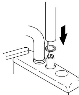
*Figure 6: Installing the Light Post*
