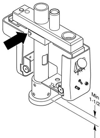
*Figure 2: Installing the Post
