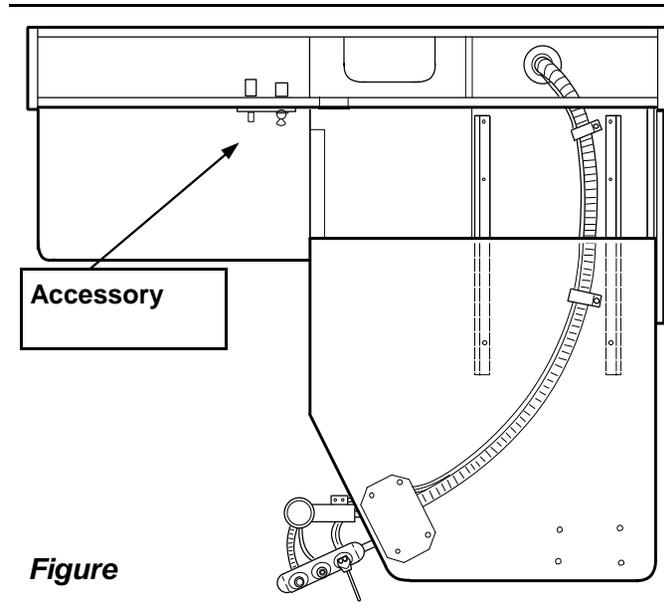
package to the underside of the counter-top. Refer to Figure 2 for orientation of the stop screw and angle of the holder bar. These two adjustments provide proper positioning of the instrument package.
