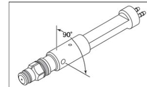
Figure 6: The Q.D. Cartridge (shut-off valve detail)
