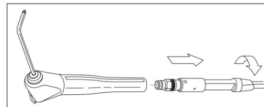
Figure 4: Syringe Removal
