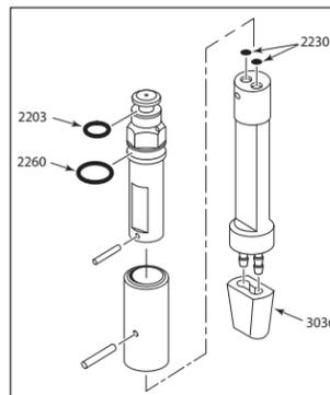
Figure 9: Cartridge Disassembly
